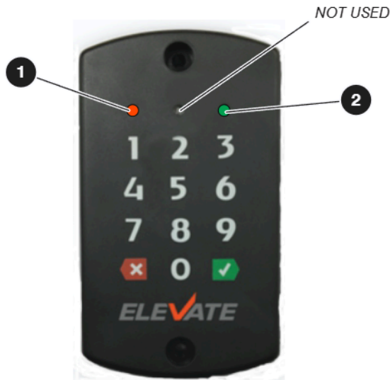
Figure 06 Keypad of the access control unit
